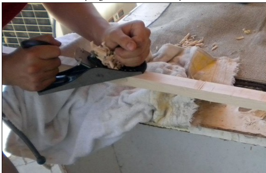
Shaping the limbs with a planar
