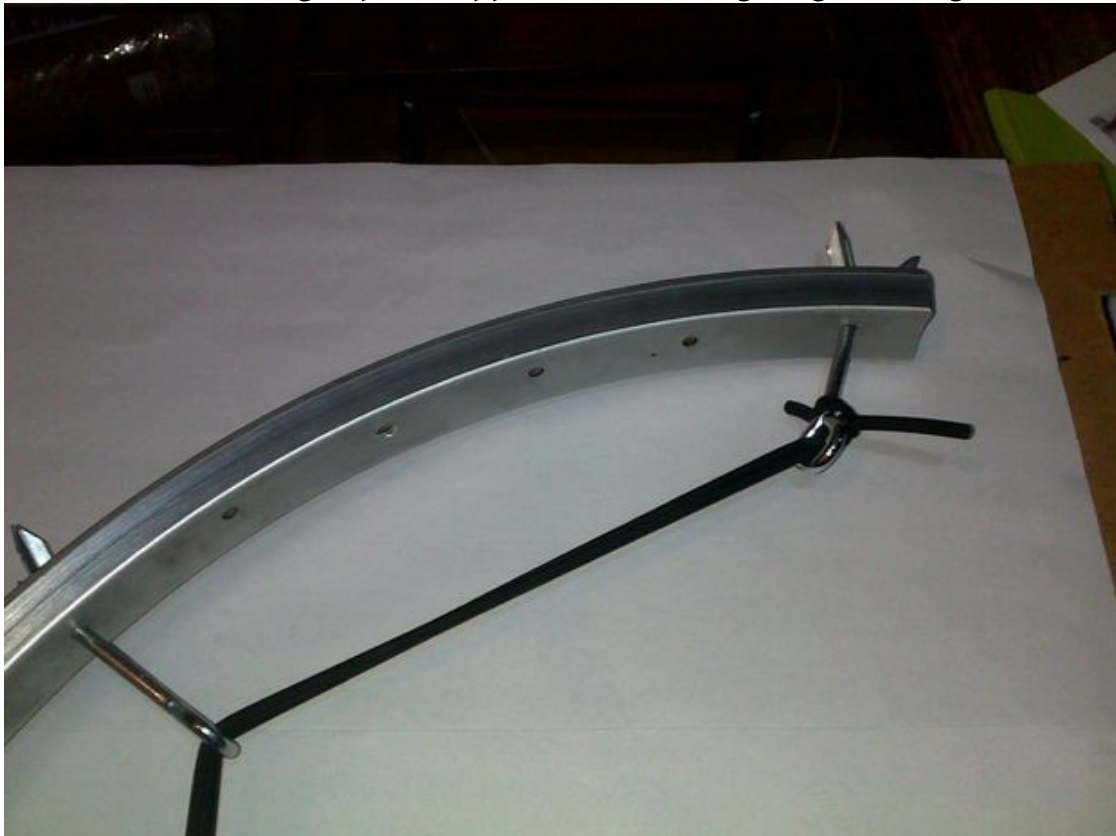
Eyelets inserted through spoke-nipple holes, holding surgical/slingshot tubing
