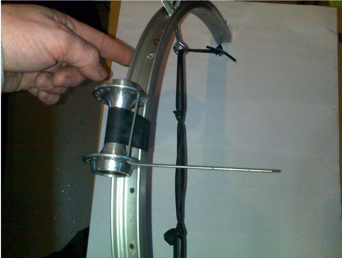
Eyelets inserted through spoke-nipple holes, holding surgical/slingshot tubing
