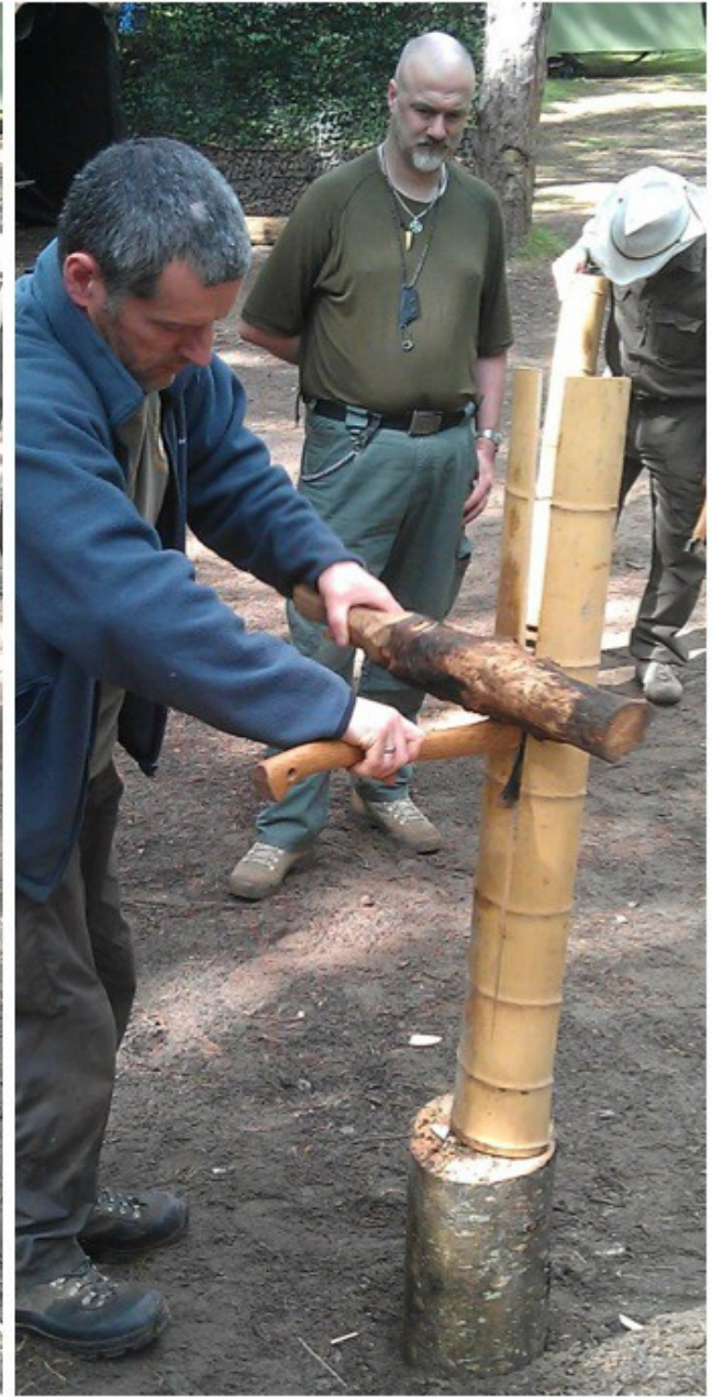
Making a Bhutanese bamboo self bow; note the thickness of the bamboo species used
