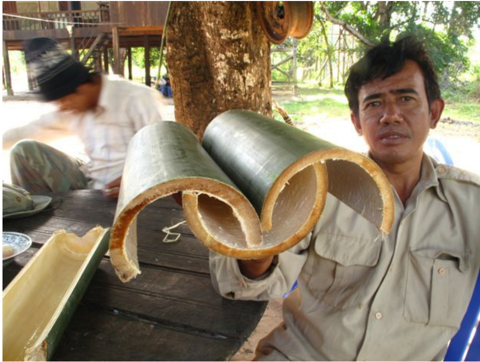
Bamboo shingles, used for weatherproof roofing
